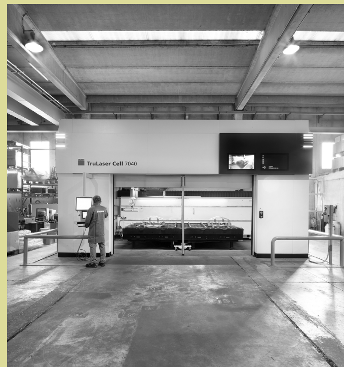
Images of the 3D fiber laser-cut machine installed at our production plant.
