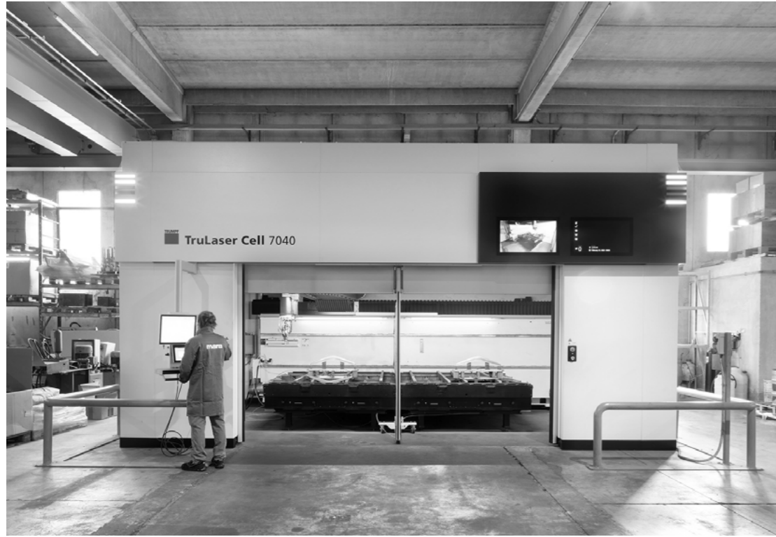
3D fiber laser-cut machine installed at our production plant.
